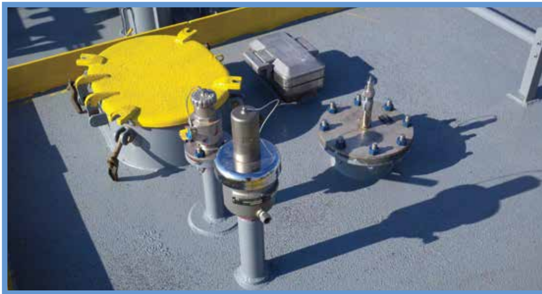
DS-39™ One Meter Rising Stick Gauge, Sampler Ball Valve, 2.5" Equate PV Valve, and SGM-1 Full View Sight Glass.
