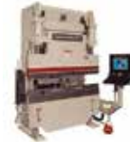
Cincinnati 90mx Maxform. Pressbrake 45 ton. 100"
