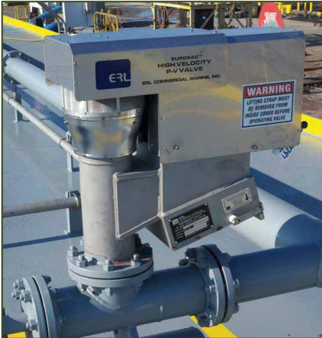
Superac 6" High Velocity PV Valve Model II mounted on collapsible vapor pipe.
