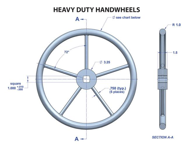
ERL's Heavy Duty Handwheels feature a stainless steel hub and spokes surrounded by a solid 1" diameter rolled 300 Series Stainless Steel ring. ERL's standard hub has a 1" square broached hole that is a full 1-1/2" thick for extra strength.
