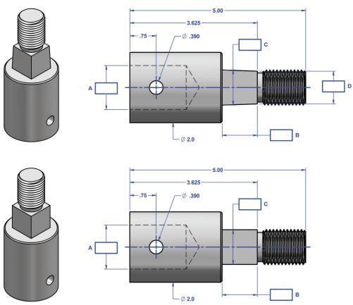
ERL stainless steel Stem Adapters are easy to use and they save you money. Class III threads and CNC machining quality insure both good fit and the ability to easily remove the handwheel without heat or destructive force. Simply weld or bolt the Stem Adapter, which has been machined to perfectly fit your handwheel, to an un-machined stainless steel bar stock for a perfect economical reach rod everytime!
