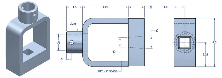
ERL's heavy stainless steel rod-to-valve connection yoke is the easiest and most economical way to connect the lower end of the Reach Rod to the Cargo Control Valve. ERL machines, from the dimensions you supply, the lower end of the Yoke to match your Cargo Control Valve stem. The upper end of the Yoke is also machined and is designed to be either welded or bolted to the lower end of the Reach Rod.
